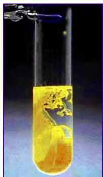
52-rasm. \text{AgNO}_3 va \text{NaJ} dan \text{AgJ} cho'kmasi hosil bo'lishi.
