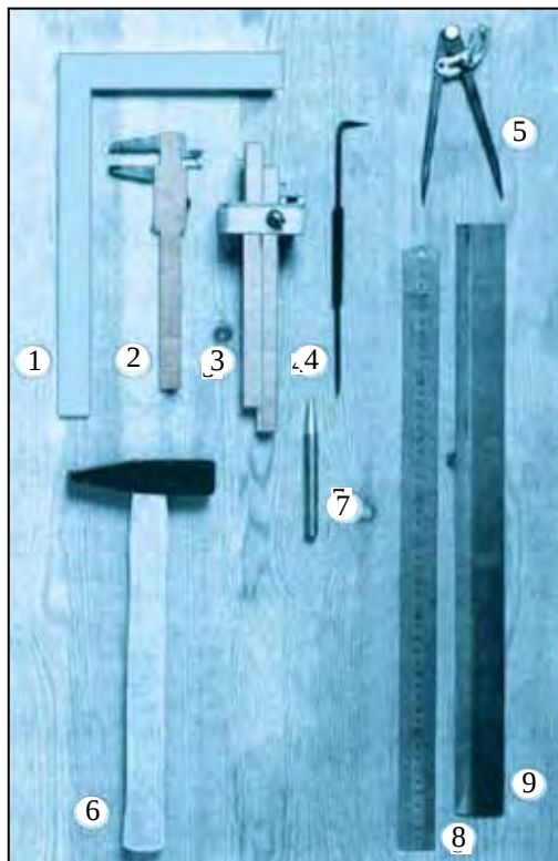
7-rasm. O'lchash va rejalash asboblari: 1–90° li burchaklik; 2–shtangensirkul; 3–masshtabli chizg'ich; 4–temir chizg'ich; 5–rejalash sirkuli; 6–chilangarlik bolg'asi; 7–kerner; 8–9–chizg'ichlar.
