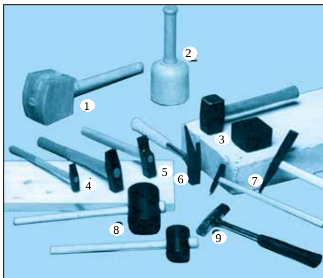
13-rasm. Chilangarlik bolg'alari va yog'och to'qmoq: 1, 2 – yog'och bolg'alar; 3, 4, 5, 6, 7 – po'lat bolg'alar; 8, 9 – plastik bolg'alar.
