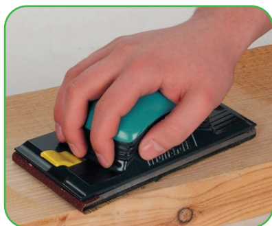
43-rasm. Jilvir qog'ozlarni mahkamlash usullari
