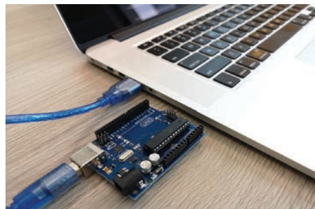
4-rasm. Dasturni Arduino UNO platasiga yozish
